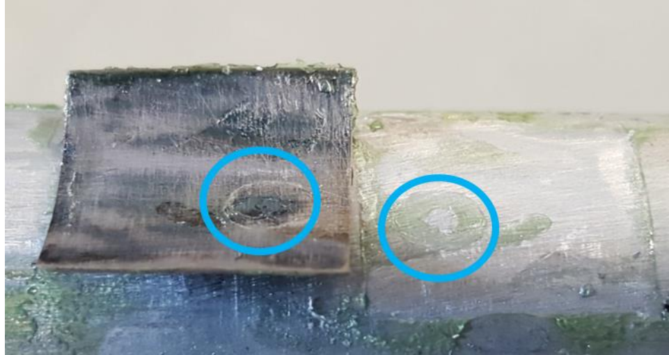
Figure 3.17: A non-uniform bond layer, with adhesive pooling around an air bubble, formed due to imperfect sanding of the shaft and shim sample.
